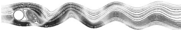
FIG. 7. Instantaneous streamlines colored by velocity magnitude. Unsteady viscous flow past a circular cylinder. Re = 200 , 256 \times 256 grid.
